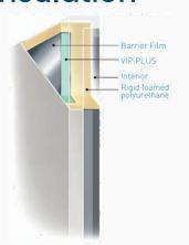
Provides up to 30% more storage capacity than a conventionally insulated freezer.
