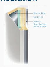
Provides up to 30% more storage capacity than a conventionally insulated freezer.
