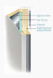
Provides up to 30% more storage capacity than a conventionally insulated freezer.
